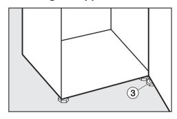
■ **Ensure** that you unscrew adjusting foot ③ from the hinge plate until it sits on the floor. Then unscrew the foot by a further 90°.
